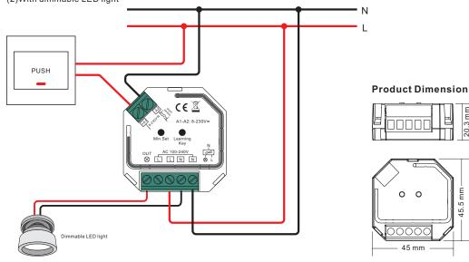
This phase dimmer adopts trailing edge dimming (reverse phase control), please make sure the connected loads support reverse phase control. Please refer to the user manual of the load or consult the supplier of the load.
